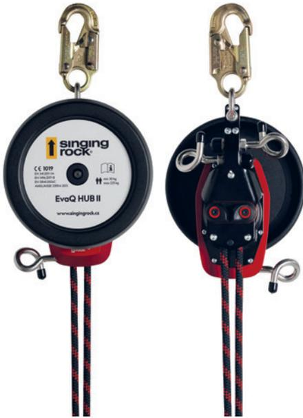
**Descender and rescue device with lifting function for height rescue by fire fighters, industrial climbers and others when exposed to a danger at great heights such as cable cars, outdoor parks, wind power plants or skyscrapers. Also suitable for quick and easy rescue and even for self-rescue of many threatened people. Certified according to EN 341:2011 class 1A (2 persons), EN 1496:2017 class B (2 persons), ANSI Z359.4:2013 (1 person), EN 12841:2006 Typ C (1 person)**
