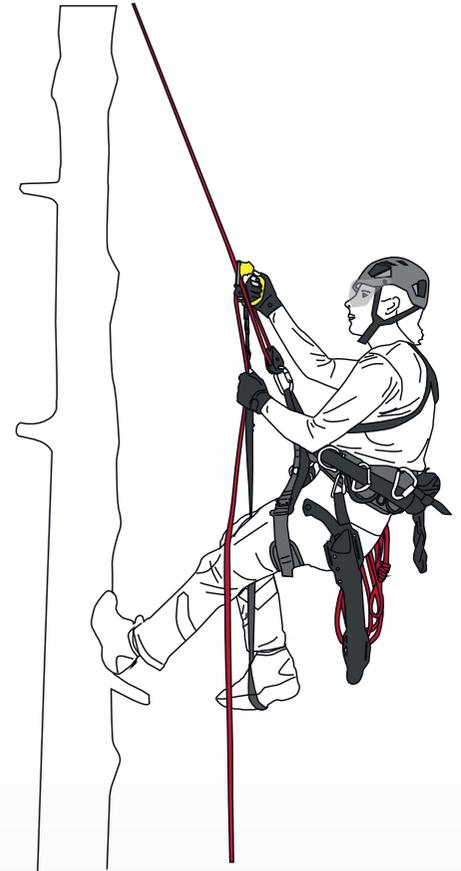
Prior to starting work, the arborist in the tree must always have two independent adjustable positioning devices.
