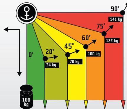
Load of continuous anchoring point. An example is creating a deviation using rope techniques.
