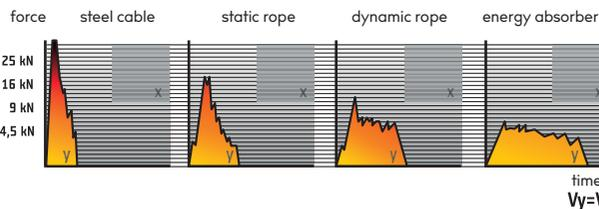
The impact force (IF) determines the maximum value of force generated during fall arrest of the object by the safety chain. The value of IP has a direct impact on the safety of worker at height. Ideally, we avoid IP if we reduce it to the lowest level possible (max 6kN)
