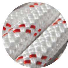
Static rope type B. Low stretch kernmantel rope of a lower performance than type A ropes, requiring greater care in use.
