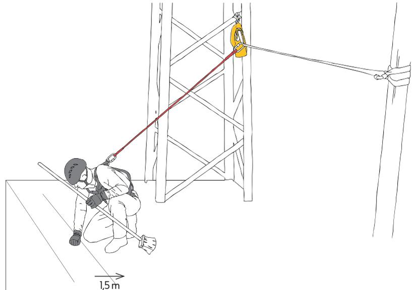
Use of mobile safety system (Fine line) to delimit safe working area
