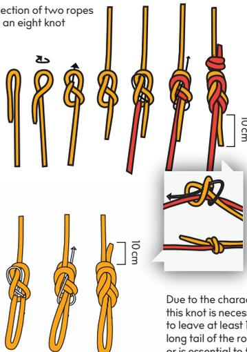
Due to the character of this knot is necessary to leave at least 10 cm long tail of the rope or is essential to tie a backup knot, double fisherman's knot
