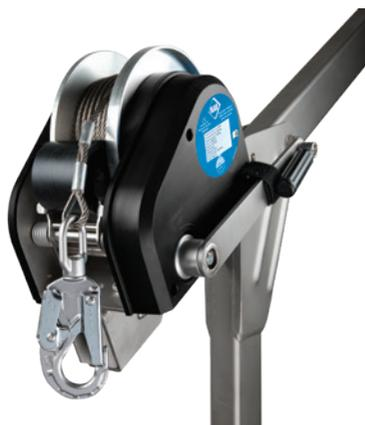
Hand crank winch for easy and jerk-free lifting and lowering of persons and loads according to Directive 2006/42/EG with 30 m stainless steel rope of  $\varnothing$  6 mm (min. breaking load 18.76 kN). SWL is 300 Kg.
