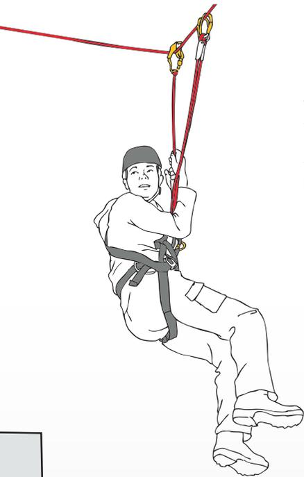
**Zip Line** At zip line the client first attaches a tandem pulley to the steel rope, behind the pulley, client attaches the first and second back up sling with the connector. The whole weight of a client is in the pulley. Back up slings move freely behind the pulley.
