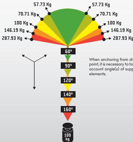
When anchoring from different point, it is necessary to take into account angle(s) of supporting elements.
