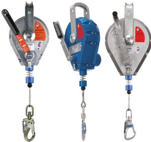
**Self-retractable arrester with built in two-way rescue/ recovery mechanism. Fall arrest device with rescue lifting and lowering facility, equipped with a recovery mechanism operated by a device mounted handle. After an arrested fall, or if the user becomes incapacitated at the bottom of a shaft, the recovery mechanism can easily be engaged by a second person to raise or lower the person to a place of safety.**
