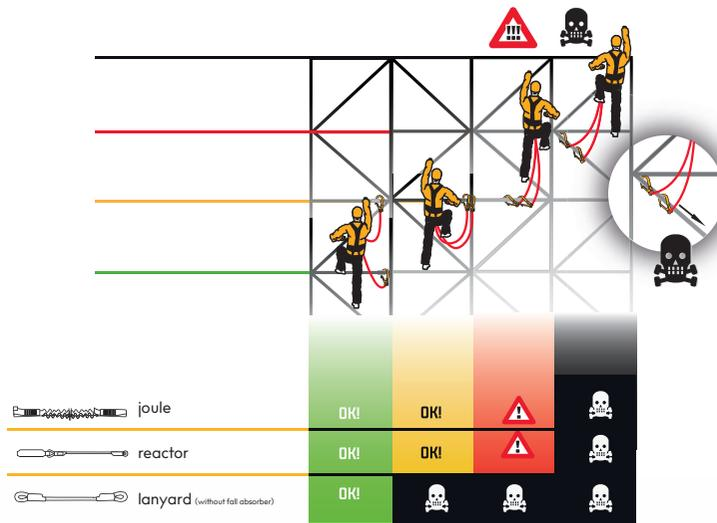
When safeguarding an ascent using a fall arrest type „Y“ it is necessary to move at the level FFI and lower. It means that the connectors (EN362) connected to the fall absorber (EN355) during the ascent do not „fall“ below the connection point of the harness (EN361) in which the absorber is connected to the harness.
