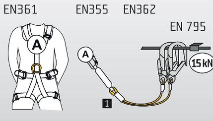
Work positioning on a frame construction
